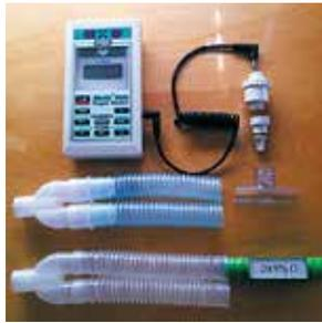
**DOXS Technology Systems**, has developed a single-use oxygen level monitoring sensor for measuring the fraction of inspired oxygen (FiO<sub>2</sub>), or the percentage of oxygen involved in the gas exchange. DOXS' technology is based on that found in zinc air batteries,
