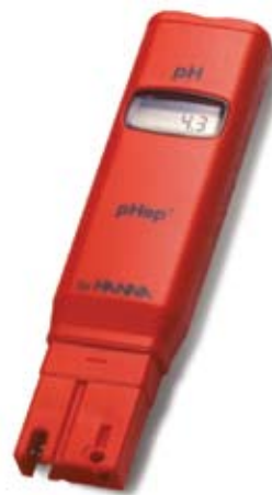
Figure 1: The pH meter's LCD display shows pH to 0.1pH resolution with an accuracy of \pm 0.1 pH. Calibration of pH could be carried out at either 1 or 2 points (usually pH 4 and 7 buffer values) quickly and easily. The electrode part is housed within the pocket sized case and is ready for use after the black plastic cap removal. The pH meter electrode was dipped in gastric fluid to measure and read the pH on the LCD display.
